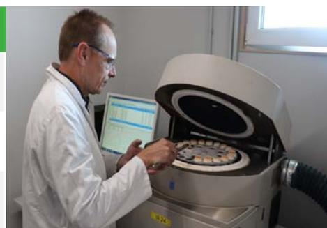
**EcoGraf** commercialisation program and pilot plant test work using a thermo-gravimetric analyser on graphite samples.
