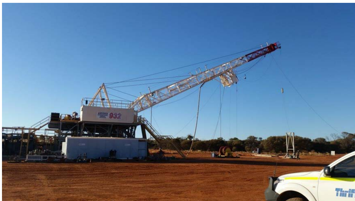
Figure 3: Ensign 932 - raising the mast at location WM26
