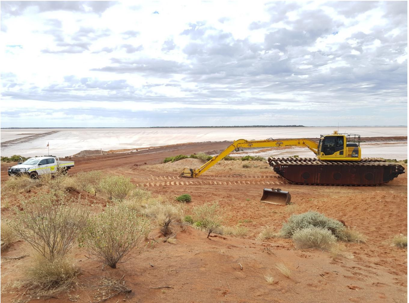
**Figure 7: Amphibious Excavator on the edge of Lake Way**
