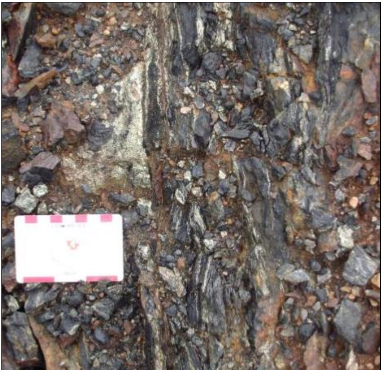
Figure 2: Banded semi-massive sulphide mineralisation in trench 2 at the Joyce River Cobalt Project
