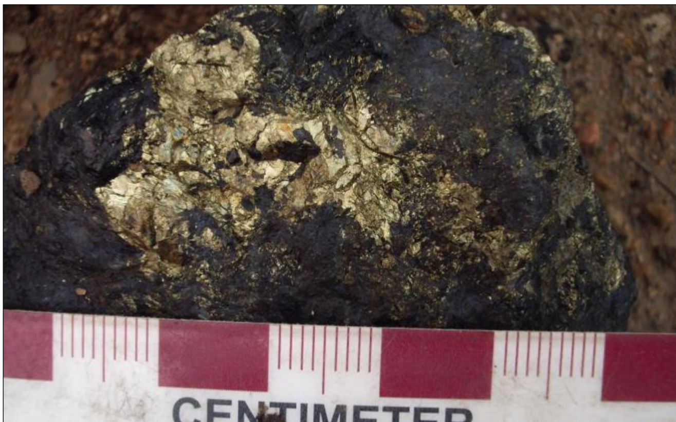
Figure 1: Chalcopyrite in pyroxenite from trench 3 at the Joyce River Cobalt Project
