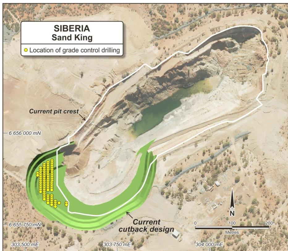
**Figure 1: Sand King Grade Control Drilling Location**
