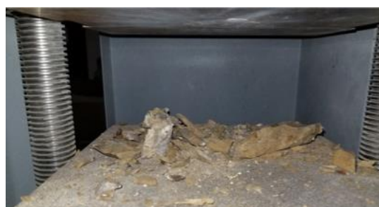
H-7 Sample 3 at UCS test completion
