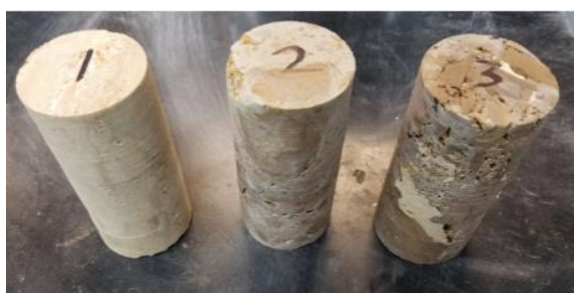
Cores of H-7 Samples before UCS test
