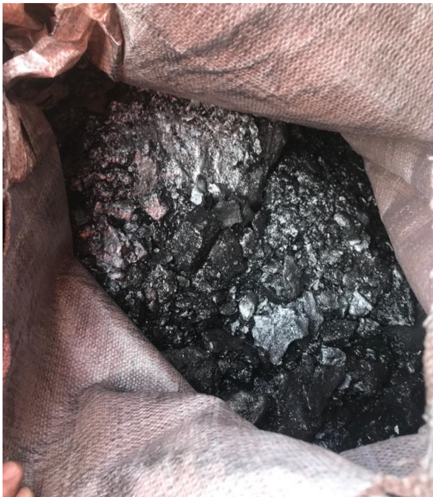
Figure 2: Wet concentrates produced from Graphmada's refurbished Process Plant.
