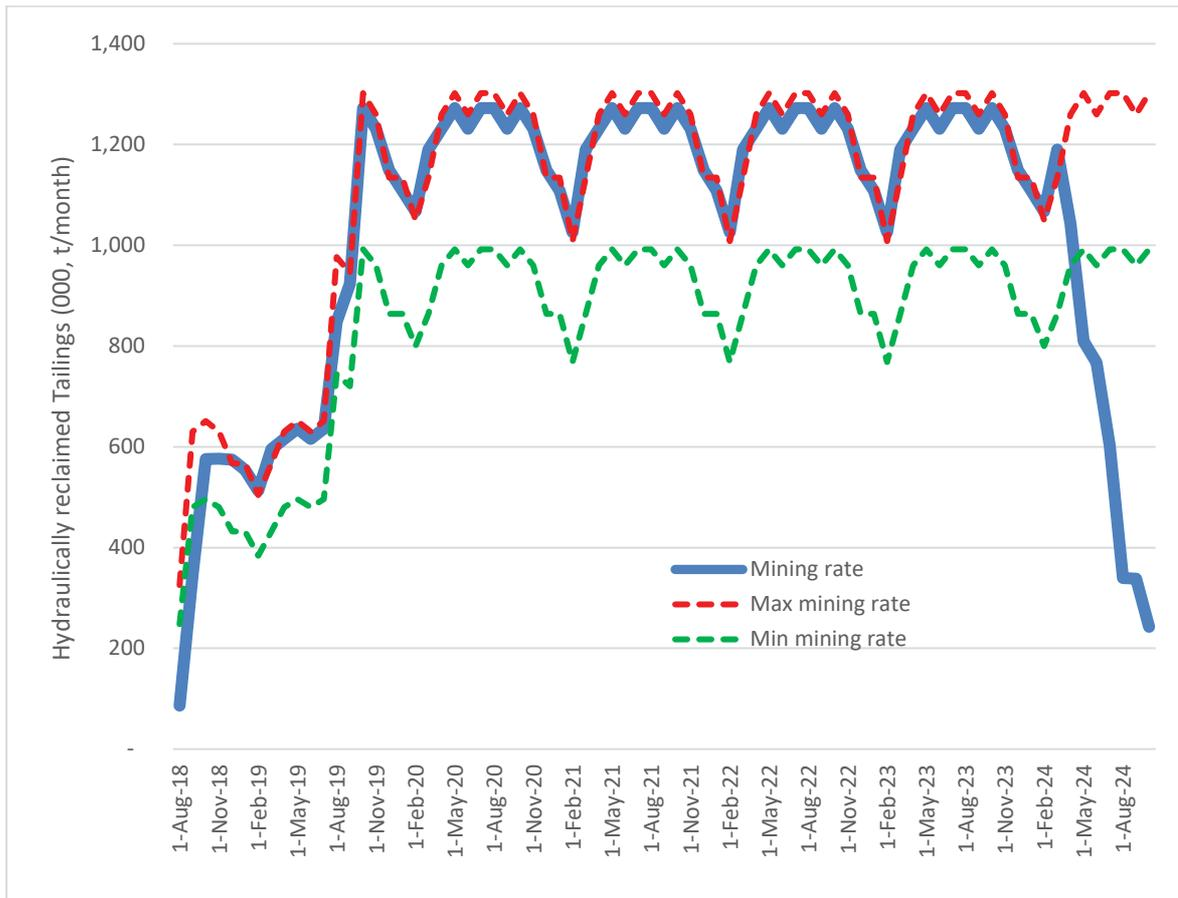
**Figure 3-1: Typical operating rates range for hydraulic mining versus proposed mining rate**
