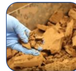
Final flotation concentrate from beneficiation pilot
