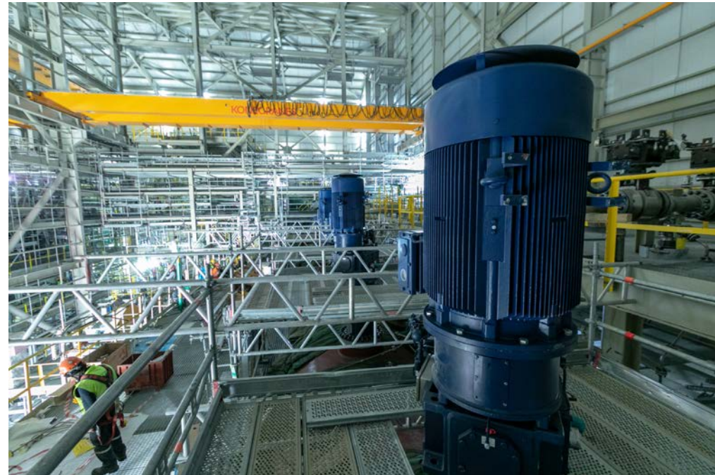
Autoclaves Showing Installed Agitator Drives
