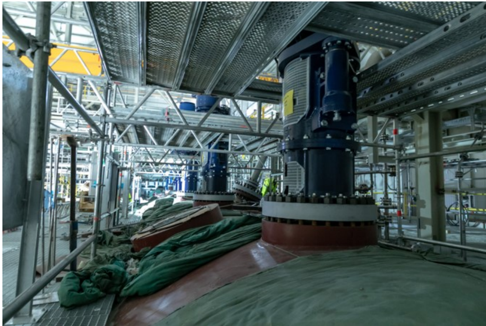
Autoclaves Showing Installed Agitator Drives
