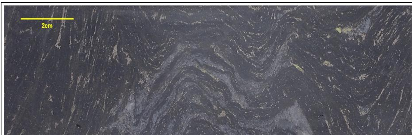
DRDD020W1 537.7m: Dark biotite altered shear fabric folded around F7 fold axis with fabric picked out by remobilised Pyrrhotite and Chalcopyrite. Intercept: 6.9m @ 18g/t fr 535m.
