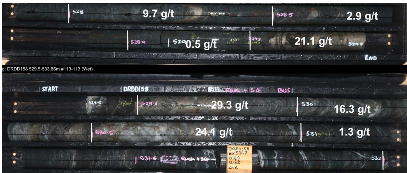
Figure 8: NEW LODGE DISCOVERY 'Viago look-a-like' west of Tribune Lode – Diamond hole DRDD167 intersection associated with ~10% pyrrhotite, trace disseminated chalcopryrite and frequent fine-grained visible gold. Assays are pending for this intersection which is located 80 metres North of DRDD170 (4 m @ 8.3 g/t gold)
