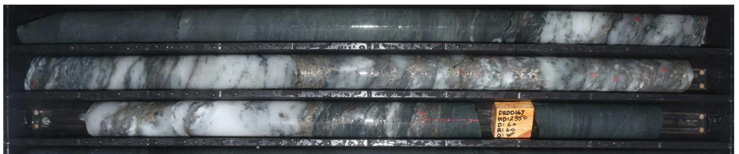
Figure 8: NEW LODGE DISCOVERY 'Viago look-a-like' west of Tribune Lode – Diamond hole DRDD167 intersection associated with ~10% pyrrhotite, trace disseminated chalcopryrite and frequent fine-grained visible gold. Assays are pending for this intersection which is located 80 metres North of DRDD170 (4 m @ 8.3 g/t gold)
