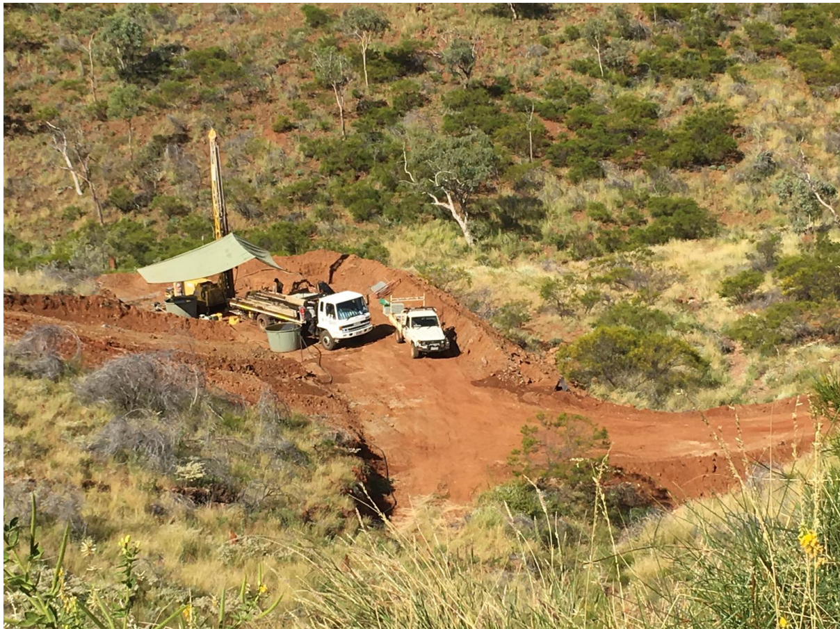
Image 1. Diamond drilling in operation targeting conductive IOCG or ISCG style mineralisation at the Mt Freda Complex that adjoins the current Newcrest Mining Limited 2019 deep IOCG drilling targets.
