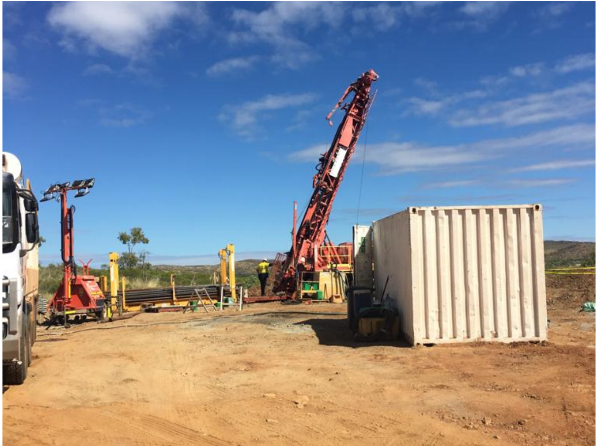
Image 7. HQ core Drilling deep IOCG or ISCG targets.
