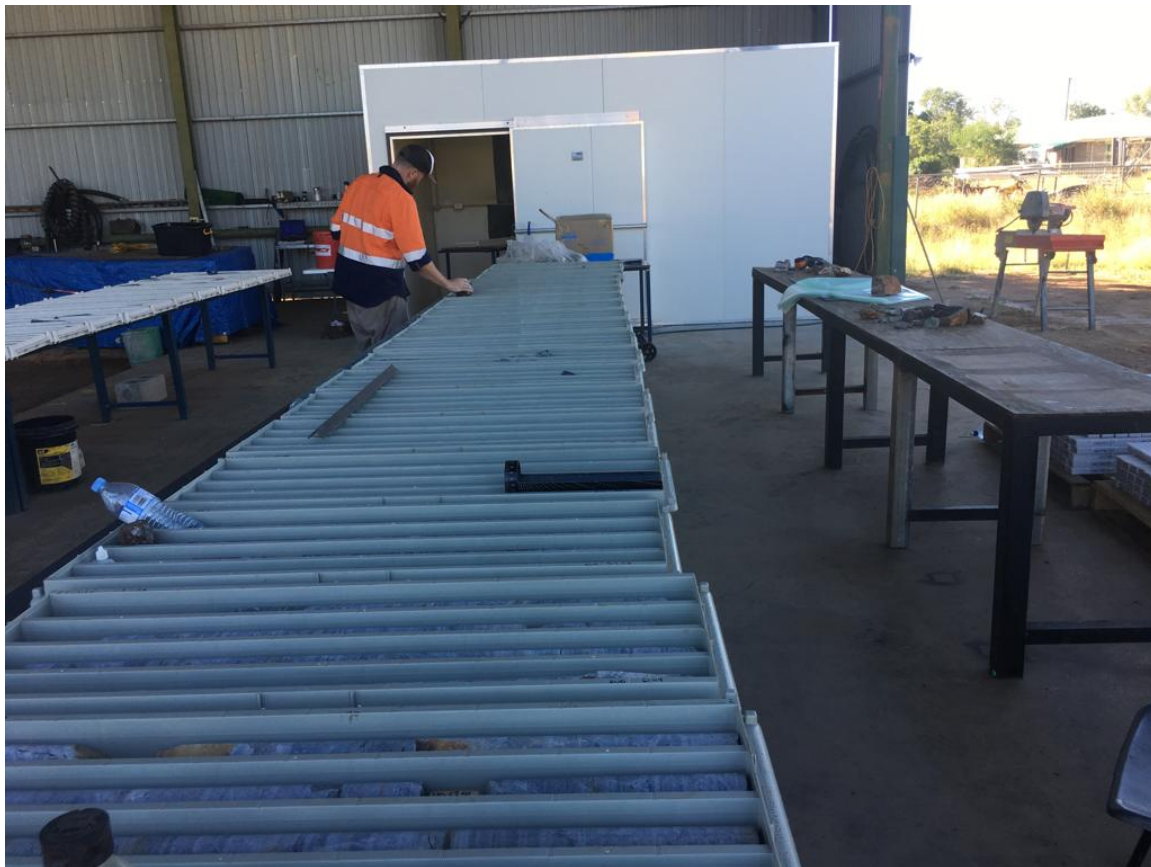
Image 6. Ausmex Geologist core logging recently drilled HQ core from the Mt Freda Complex. Core will be logged, cut, sampled & dispatched to ALS laboratories in Townsville, within initial core assays anticipated to be completed by late June.
