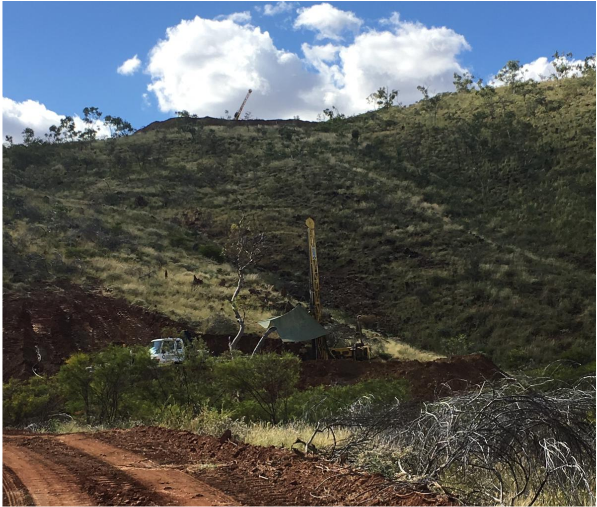
Image 9. HQ core drilling Large IOCG or ISCG conductive targets in progress, Mt Freda Complex.
