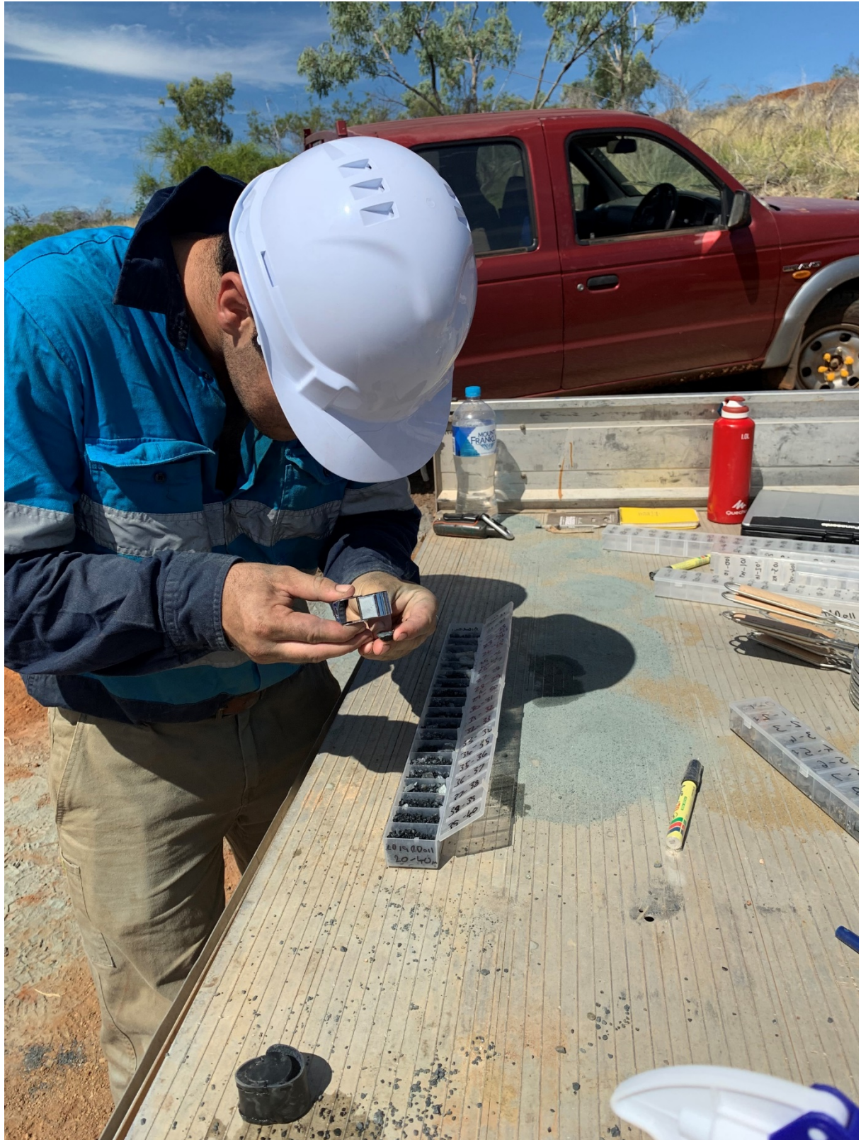
Image 3. Ausmex Geologists logging RC drilling chips from the Golden Mile, where the Company is focusing on defining shallow, high grade gold mineralisation suitable for a bulk mining, open cut operation.
