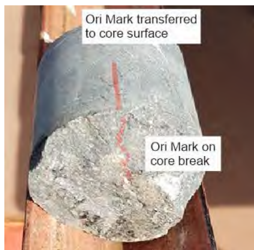
Figure 9.2 Example orientation mark on drill core
