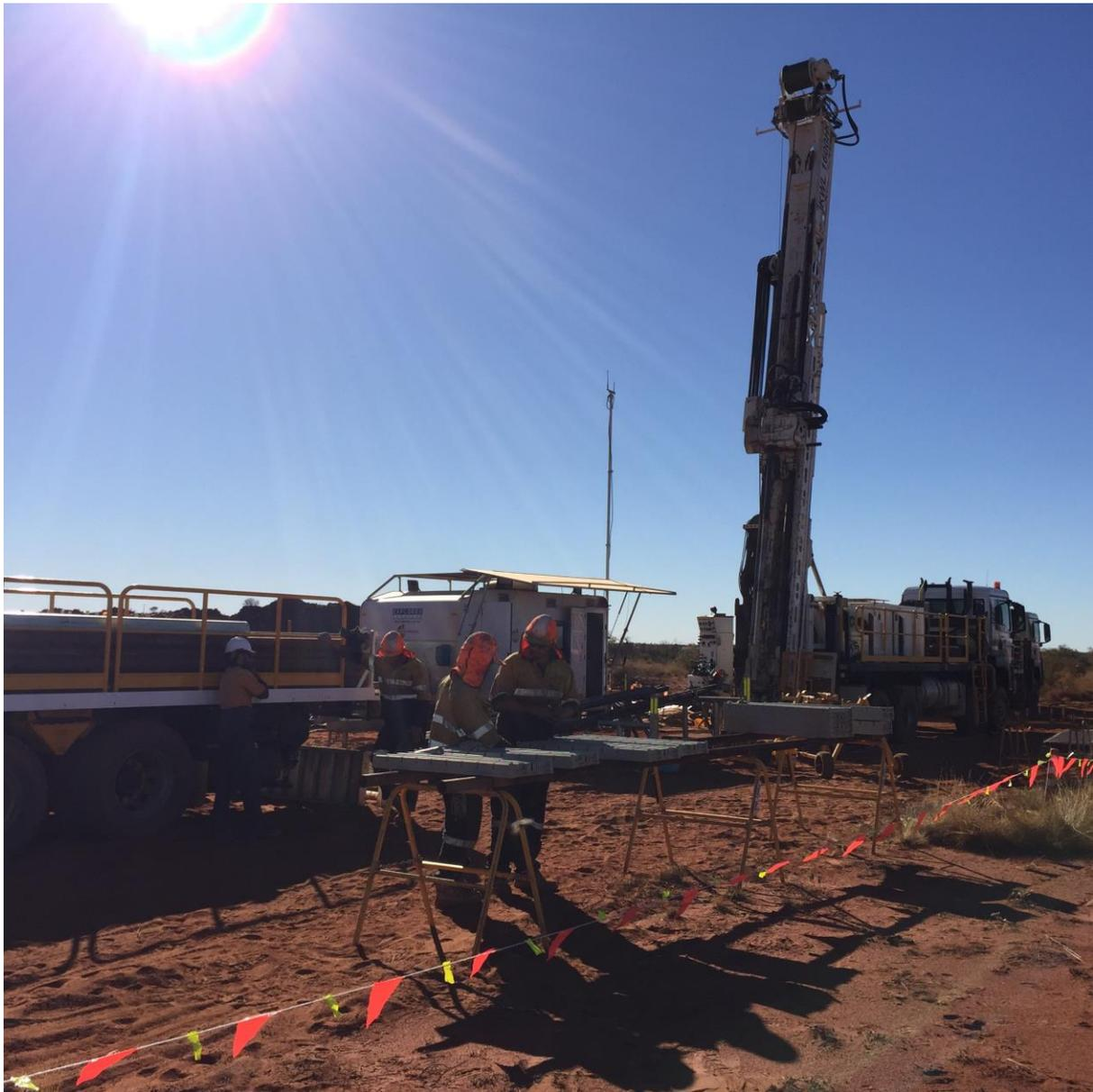
**Figure 1.** Geologist logging core from historic first drill hole into the large North Dovers IOCG target.
