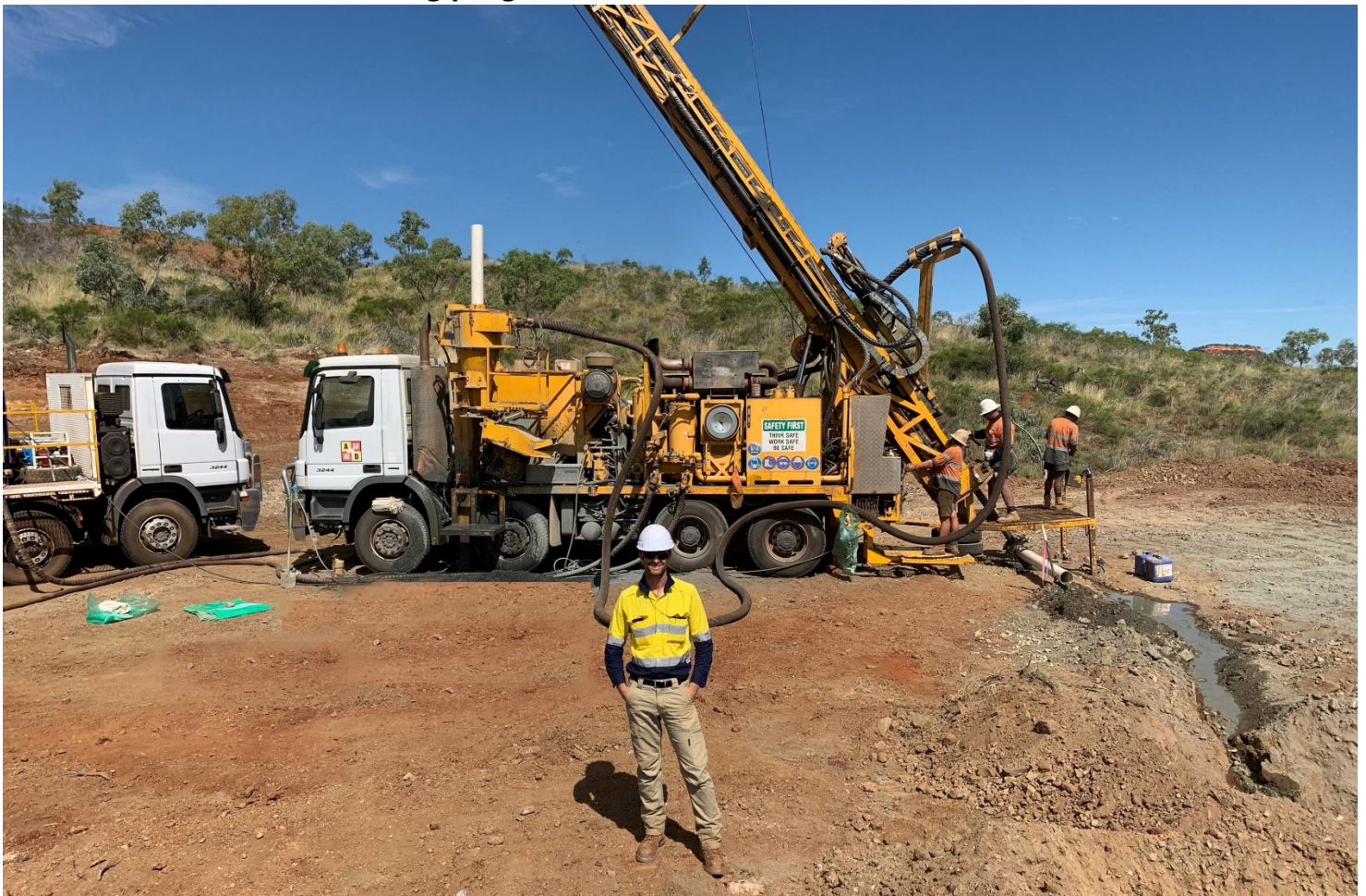
Image 1. QLD Exploration Manager Kieren Whittock supervising RC Rig 1, pre collar drilling for deep diamond drilling targeting IOCG style mineralisation at the Mt Freda Complex.
