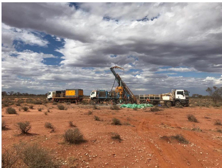
RC Drilling at King of the West
