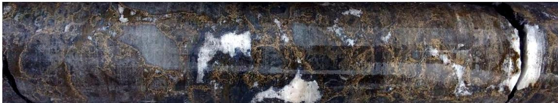
*Image: Diamond Core From AF013, 124.0m. Example of Abundant Sphalerite (Pale Brown) in Matrix of Dolomite Breccia Occurs Over 4m<sup>1</sup>.*
