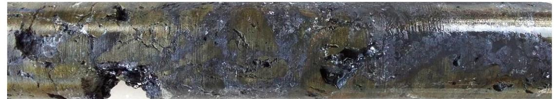
*Image: Massive Sulphides – Typical Galena (Grey-Blue) With Pyrite (Bronze Colour), Diamond Core from AF005, 82.1m. Strong Lead Mineralisation is Intersected over 9.4m Length in this Particular Hole<sup>1</sup>.*
