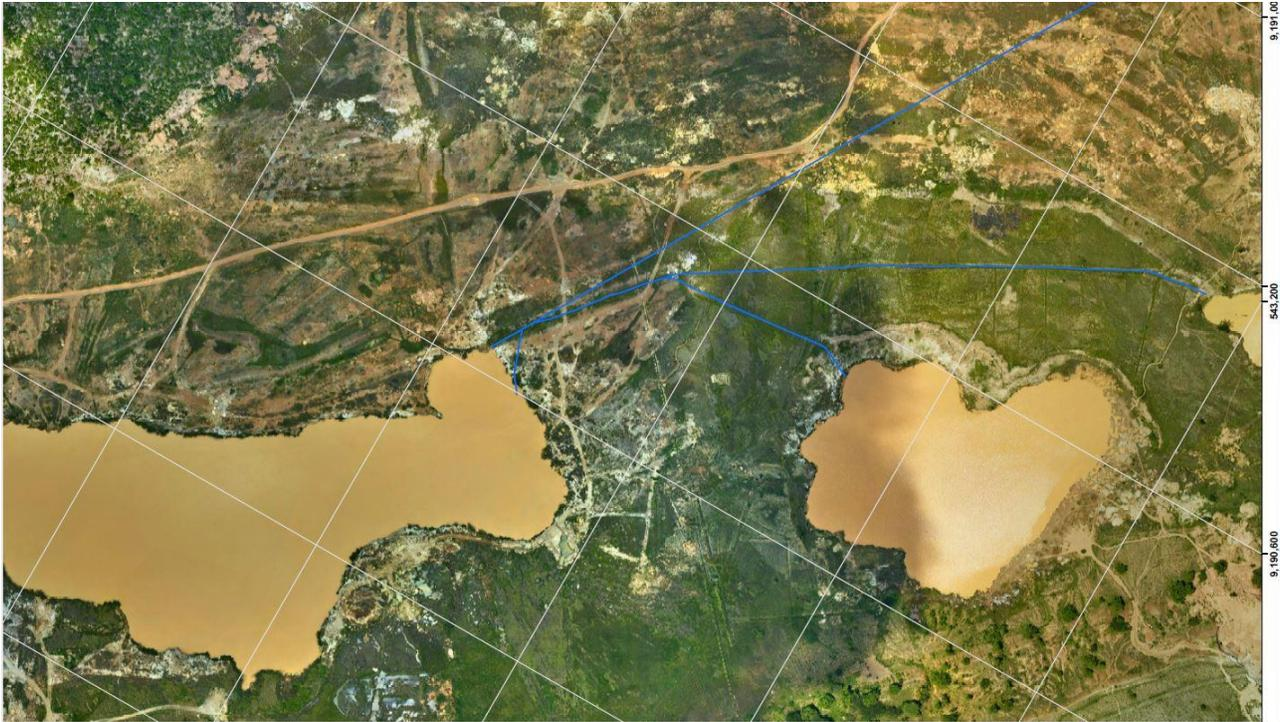
*Figure 1. Existing and newly renovated dewatering channels (blue) heading N-E from the Roche Dure open pit*
