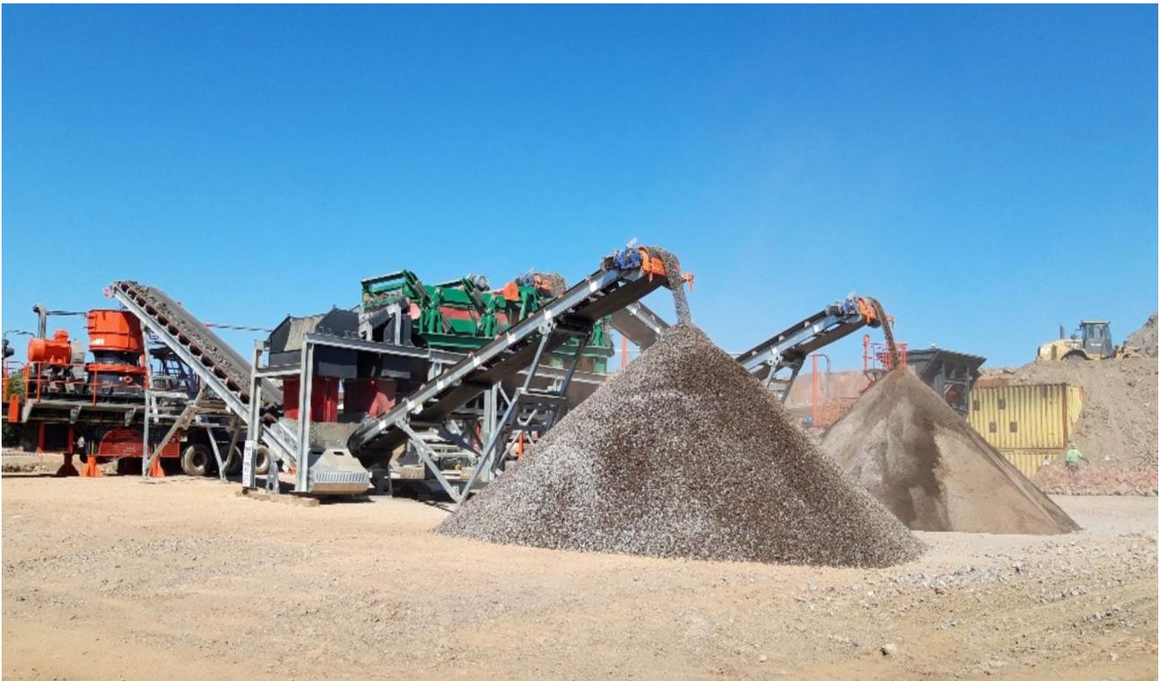
**Figure 1: Semi-permanent 400tph contract crusher in operation.**
