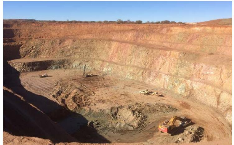
**Photo 1: Matilda M1 cutback nearing completion 68m below surface approaching strong ore zones**
