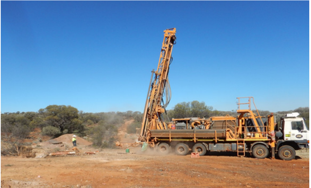
Figure 5. RC Drilling at Bell Chambers Gold Project
