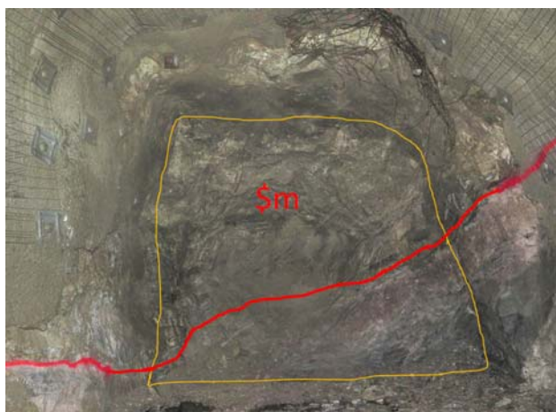
370 west ore drive (4.5m W x 4.5m H) with a face grade of 5.1% Ni
