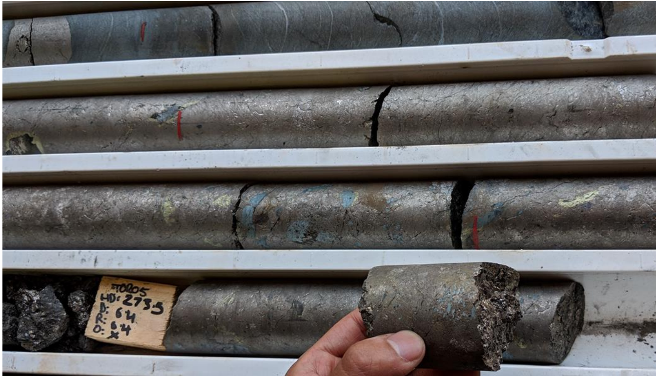
Figure Four | Massive Sulfides in TOR05 from drilling at the Thor Prospect.
