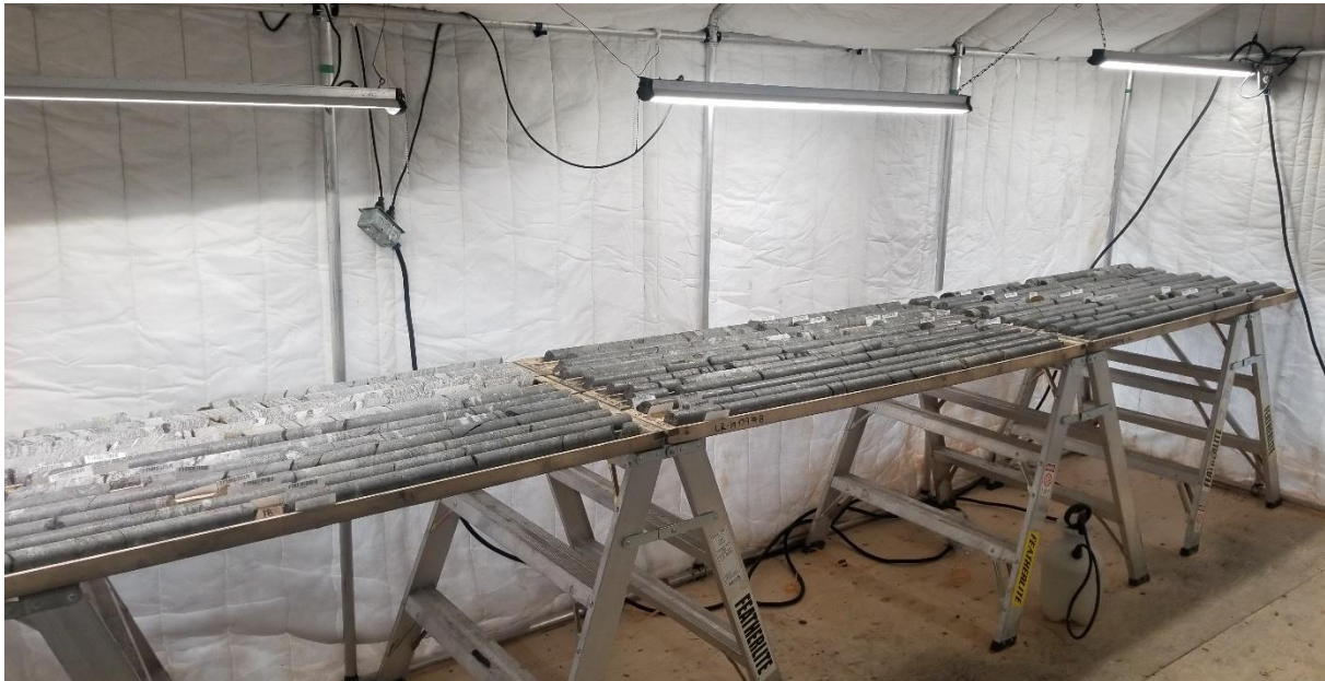
Figure 2: Drill core of DDH LR19-09 which intersected the Graphitic Carheil Zone over an extensive thickness of 75.2m (apparent thickness) from a depth of 9.5m to 84.7m
