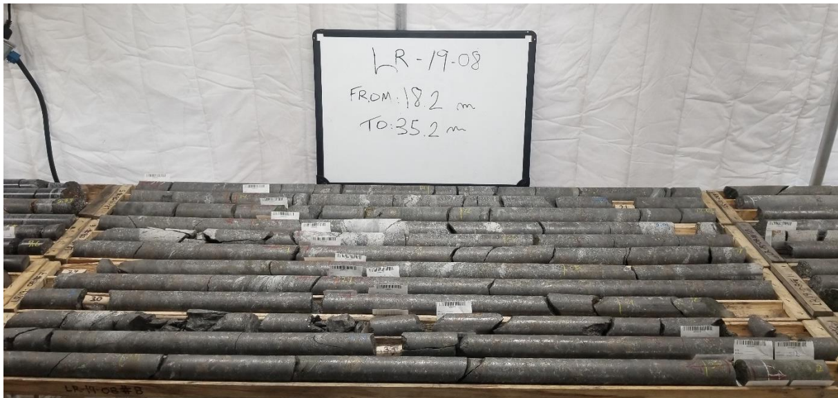
Figure 3: Drill core of DDH LR19-08 which intersected a zone of semi-massive graphite mineralisation corresponding with the Main Graphitic Carheil Zone. The drill core shown in the image represents an intersection of 17.0m ( apparent thickness ) from a depth of 18.2m to 35.2m, which is contained within a larger intersection of 47.72m ( apparent thickness ) from a depth of 7.83m to 55.5m
