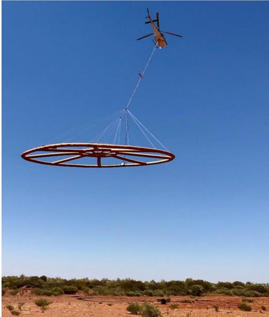
Figure 2 AEM Survey Helicopter in action
