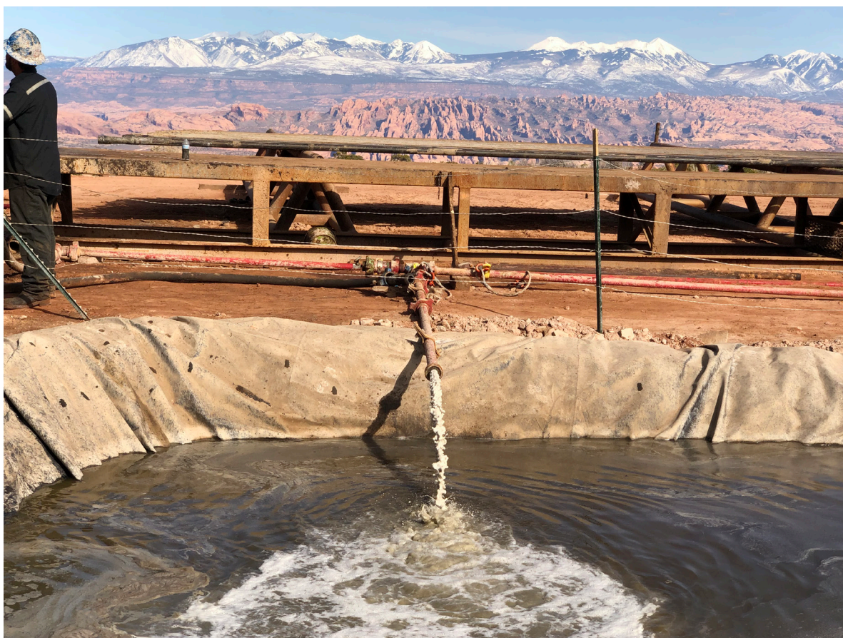
Figure 1: Supersaturated brine free flowing direct from the Long Canyon No. 2 well to the cuttings pit.
