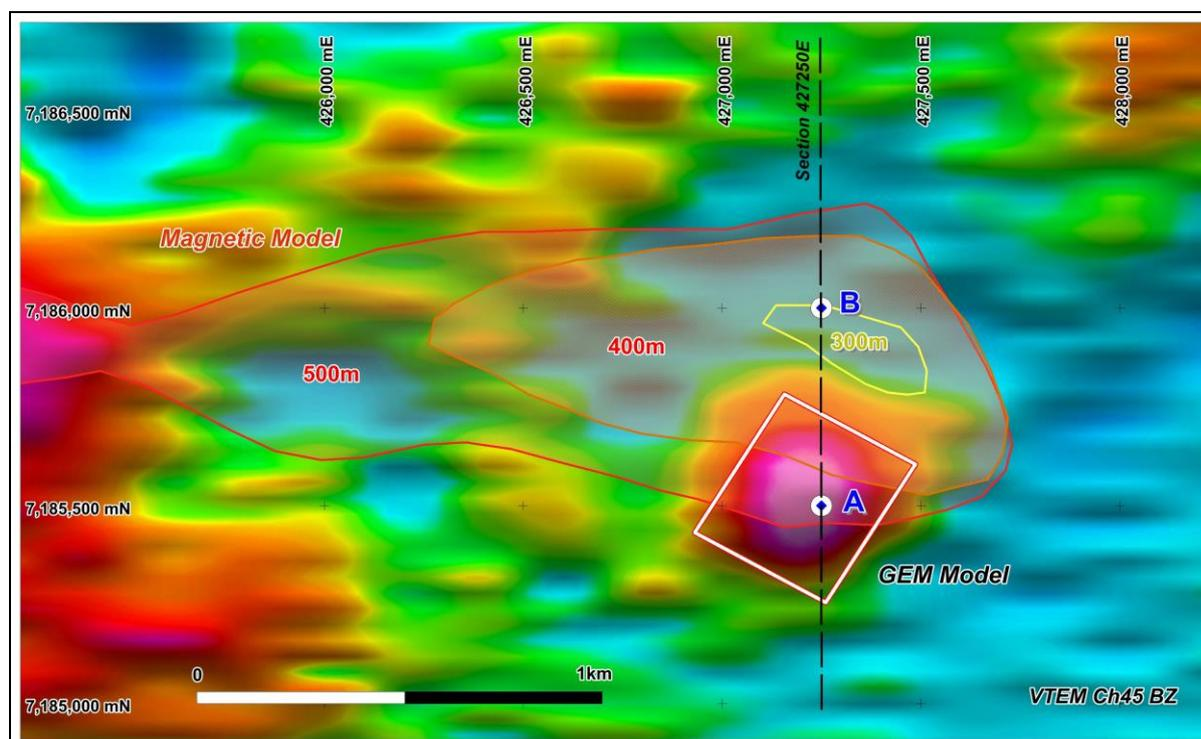
Figure 1: Yallum Hill EM and magnetic models showing planned drill-holes.
