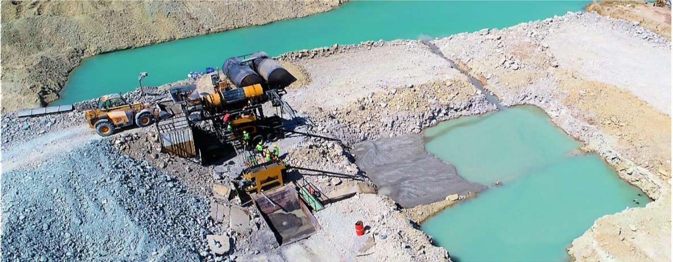
**Figure 11.** Macy 1st Jig Wash Processing Plant
