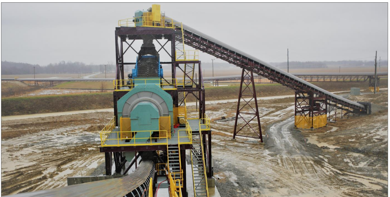
Figure 4: Raw coal reporting to the CHPP ROM screen and rotary breaker
