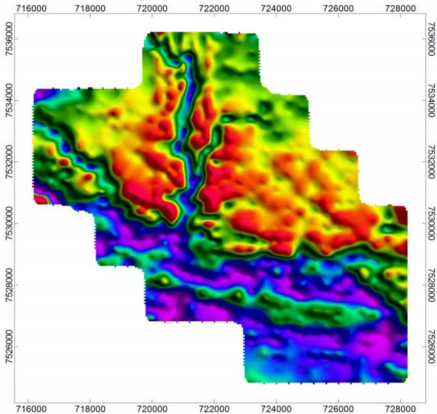
Figure 2a. First Vertical Derivative (vertical rate of change) Gravity contours in mgal over EL24808, modelled with basement at a nominal density of 2.67
