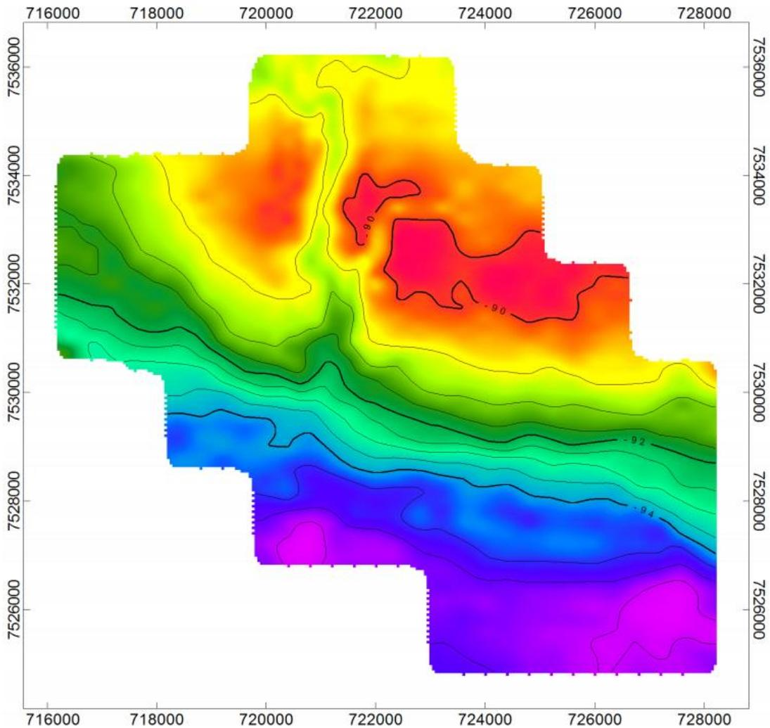
Figure 1a. Gravity contours in mgal over EL24808, modelled with basement at a nominal density of 2.67.
