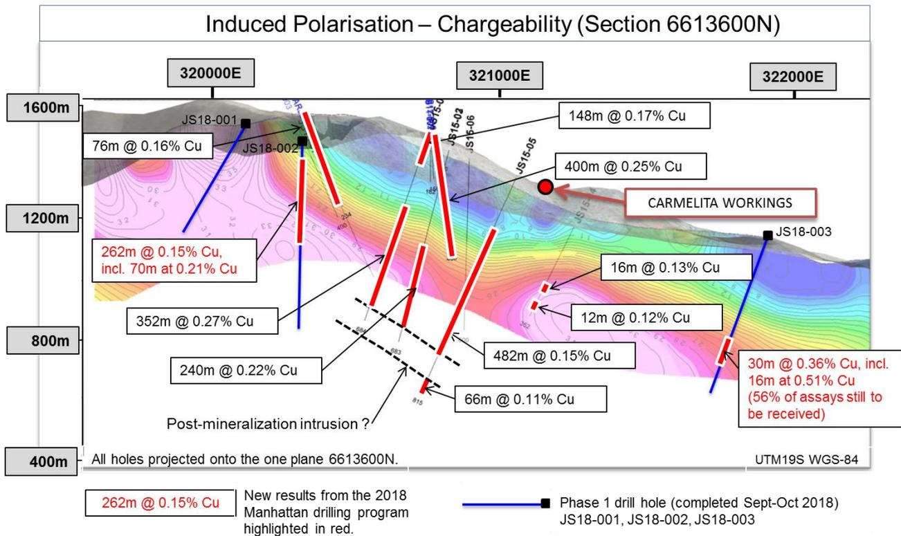
Figure 3 | Drill section showing imaged IP Chargeability and all mineralised drill results (2011, 2012, 2015, 2018) projected onto section 6613600N (UTM19S WGS84). Manhattan holes JS18-004 (completed) and JS18-005 (in progress) lie off this section 600m and 1,100m respectively further to the northeast.
