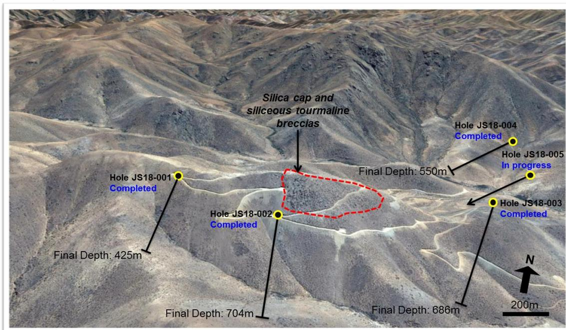
Figure 1 | Relative positions of 2018 drill holes (completed and in progress) at Joshua shown on north-looking Google image.
