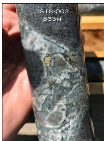
Figure 2 B. Hydrothermal dacite breccia with albite rims on biotite-magnetite altered breccia clasts and with a sulphide-bearing chlorite matrix (hole JS18-003, 533m).
