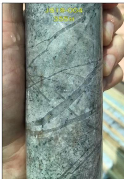
Figure 2 A. | Silicified dacite porphyry containing molybdenite-bearing A-type quartz veins (hole JS18-004, 355m). Assays awaited.
