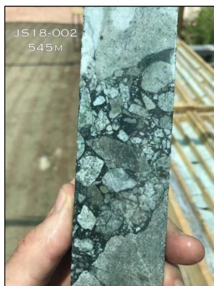
Figure 2 D. Sulphide-bearing hydrothermal dacite breccia with tourmaline matrix (hole JS18-002, 545m).
