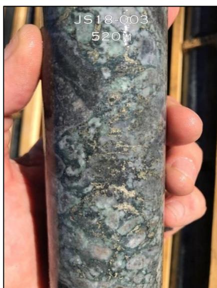
Figure 2 C. Hydrothermal dacite breccia with albite rims on breccia clasts and sulphide-bearing silica-chlorite matrix (hole JS18-003, 520m).
