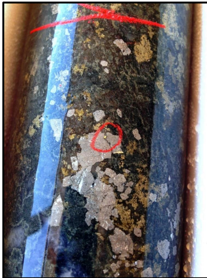
Figure 5: Hole 18SARD004, showing spectacular arsenopyrite associated with high grades and visual gold at 139m down hole. Assays returned 1.32m @ 7.90 g/t Au, drill core diameter is 6.5cm
