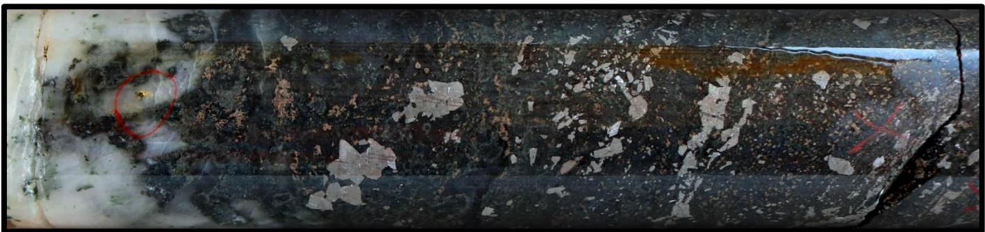
Figure 6: Hole 18SARD023 showing visual gold in quartz and arsenopyrite. Assays pending, drill core diameter is 6.5cm
