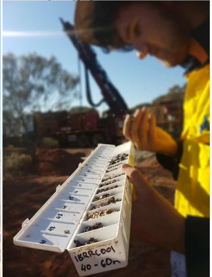
NTM Geologist logging the first RC hole at the Hub
