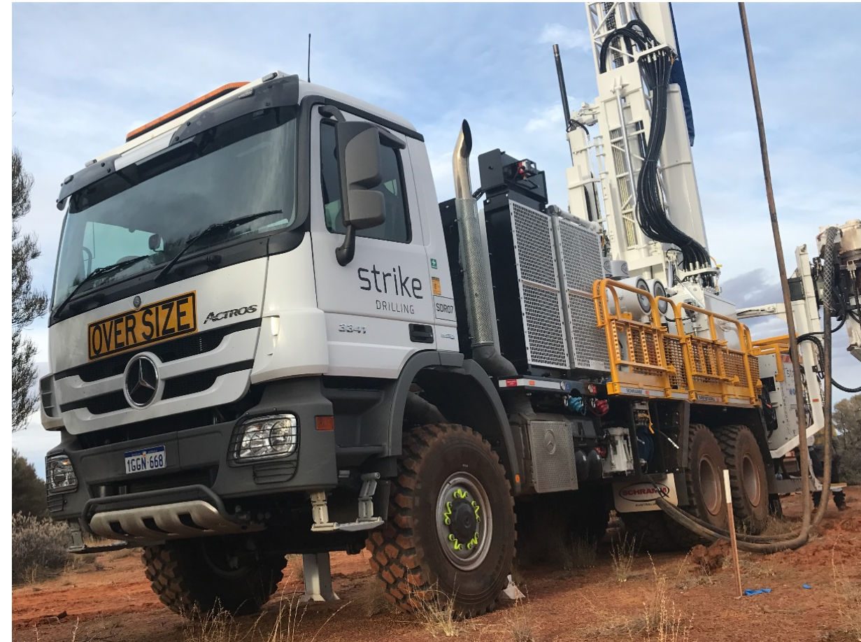
New multi-purpose Strike AC/RC rig (5,500m planned)
