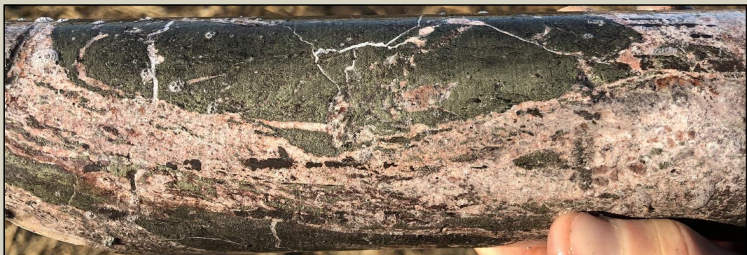
Anhydrite-pyrite-chalcopyrite vein at 589m.
