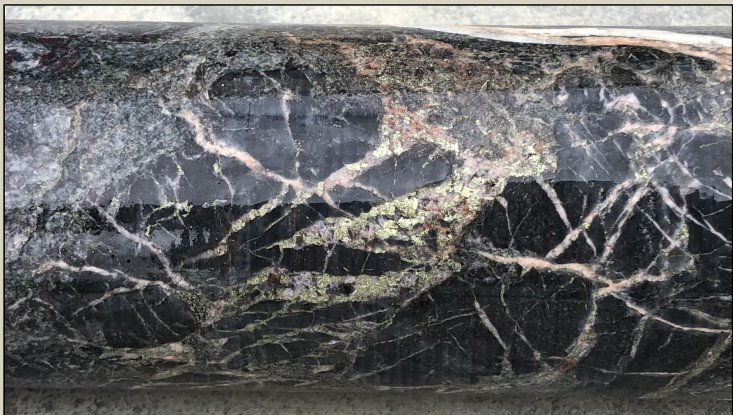
Anhydrite stockwork veining with well-developed chalcopyrite at 622.6m
