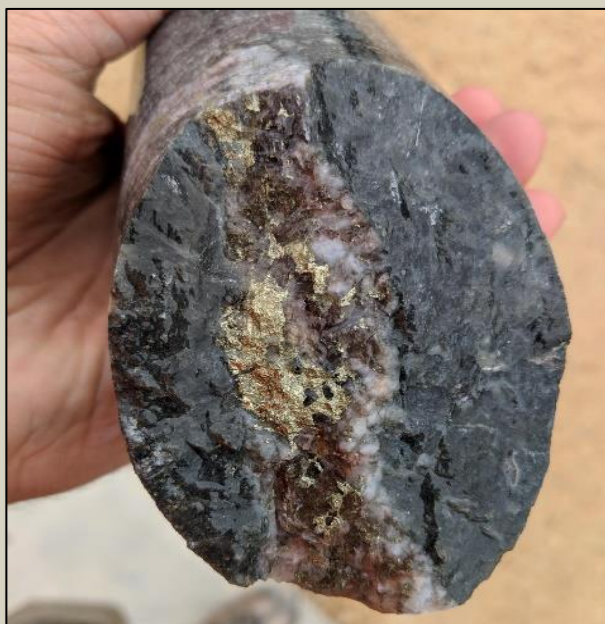
Quartz Anhydrite vein with chalcopyrite mineralisation at 689.7.
