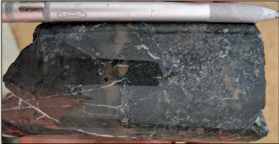
Breccia with magnetite/hematite alteration and chalcopyrite mineralisation at 692m.
