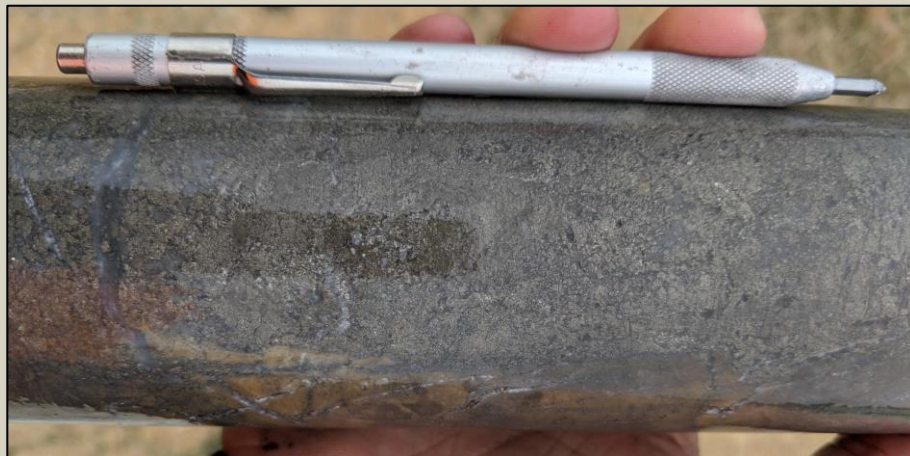
Massive pyrite vein with sericite / ankerite alteration at 734.4m.
