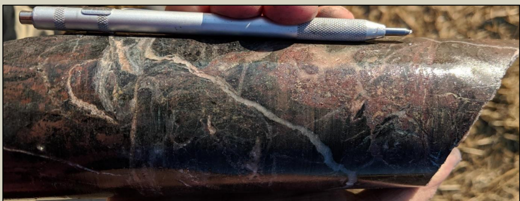
Andesite hosting well developed hematite/magnetite alteration and disseminated chalcopyrite at 592.3m.
