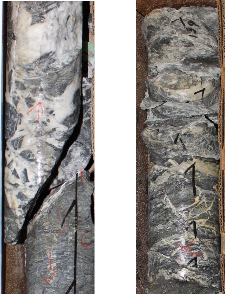
Figure 3. Hydrothermal Brecciation and Veining, Brecciation and Alteration in meta chert – Hole 7
