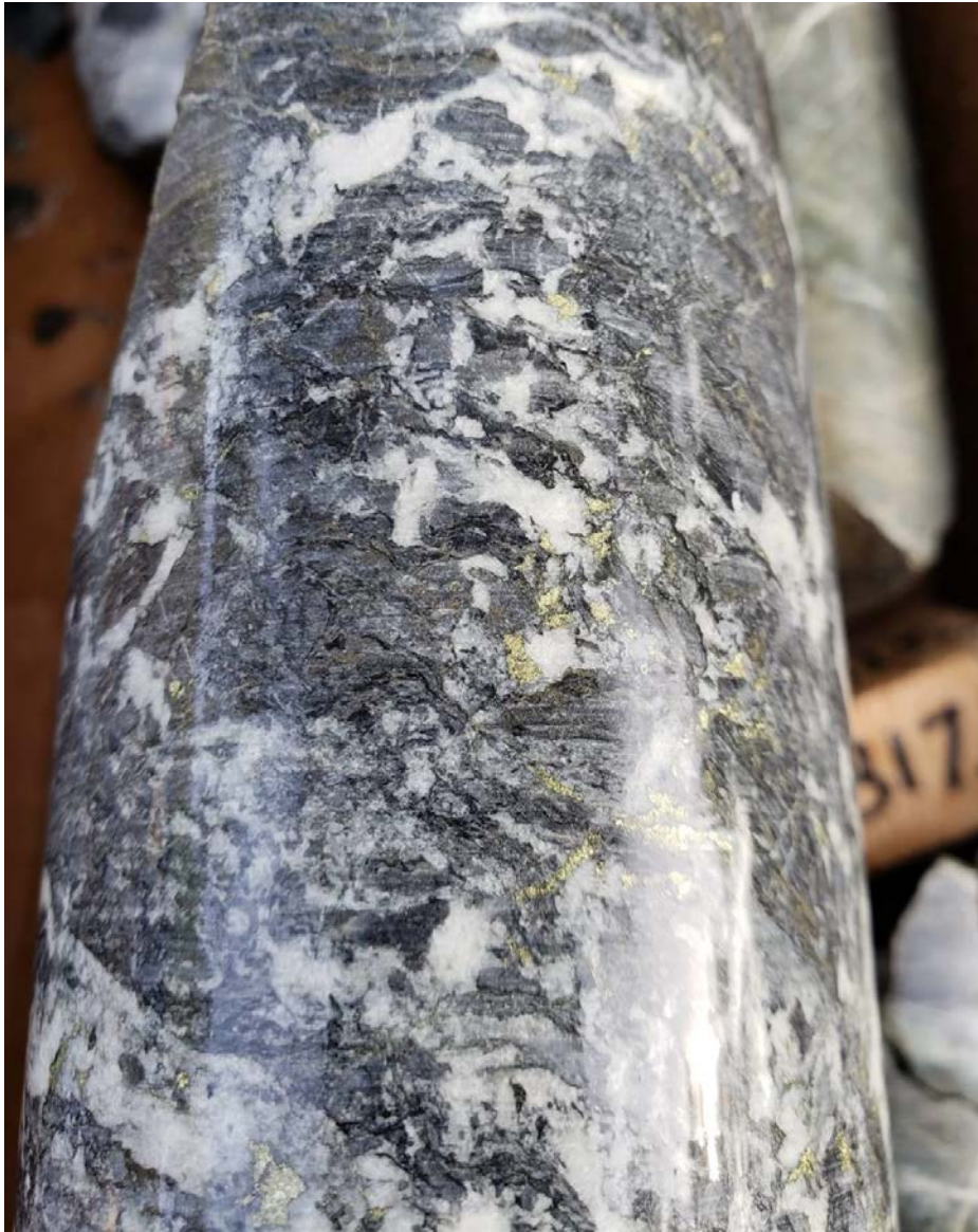
Figure 2. Quartz-Carbonate Breccia with disseminated chalcopyrite – Hole 5
