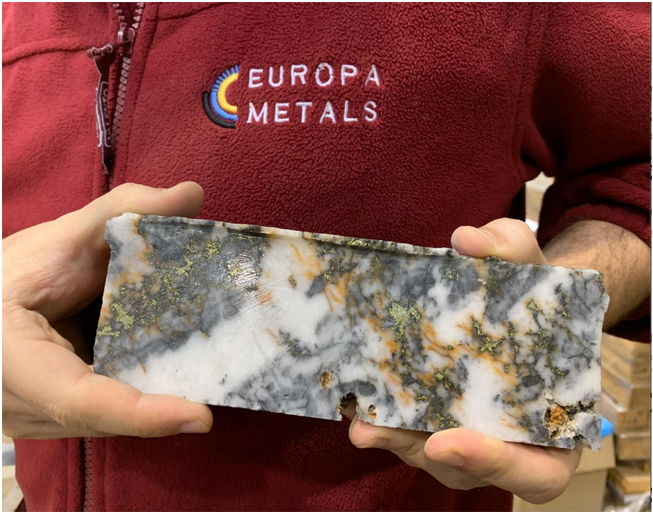
Image 1: TOD-020 drill core with highly visible chalcopyrite copper sulphide mineralisation
