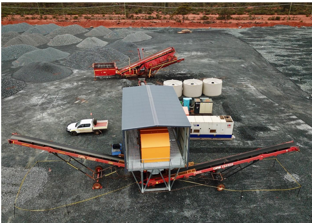
Figure 3: Typical on-site sorting layout (Steinert sorting machine in the centre)
