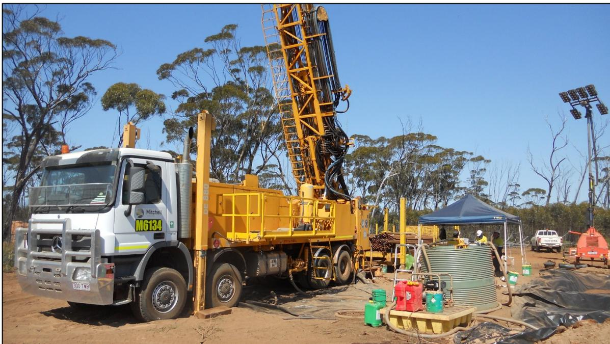
**Figure 3: Commencement of diamond drill hole PLJD004 to test the modelled extension of Abi Rose nickel mineralisation**
