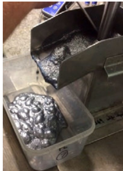
Figure 2b - High grade (47-64%) lead concentrate produced by the 2 nd cleaner stage of test AF8.
