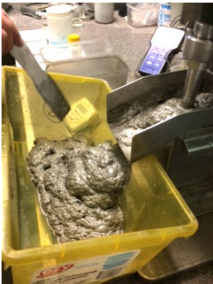
Figure 2a - High grade (54-59%) zinc concentrate produced by the 2 nd cleaner stage of test AF8.
