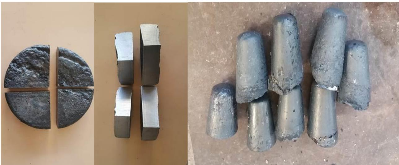
Figure 1: Pictures of sectioned final crude steel disc and cast ingots (Source: Tenova)
