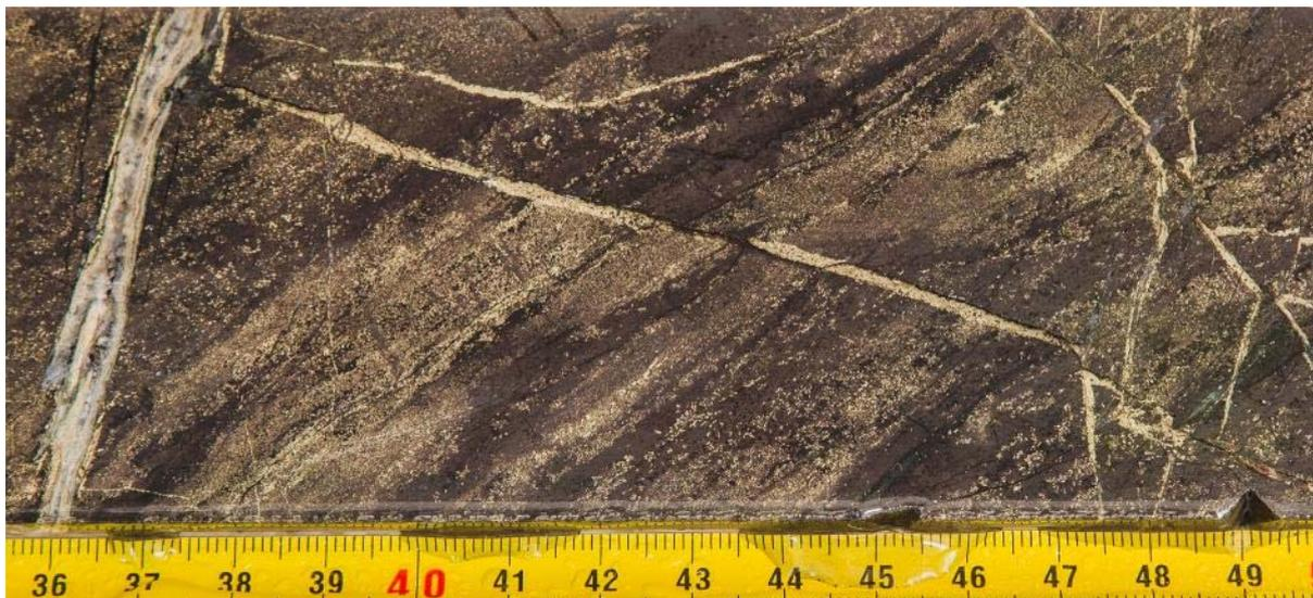
**Figure 1.** Visible copper sulphides and magnetite in half-core, hole ZX-18025, 93.9m down-hole depth. Copper sulphides comprise mainly chalcopyrite (yellow colour). Assays returned mineralisation grades of 5.4% Cu, 3.7g/t Au and 16.3g/t Ag for the interval including the above core-photograph. Scale bar is in cm.
