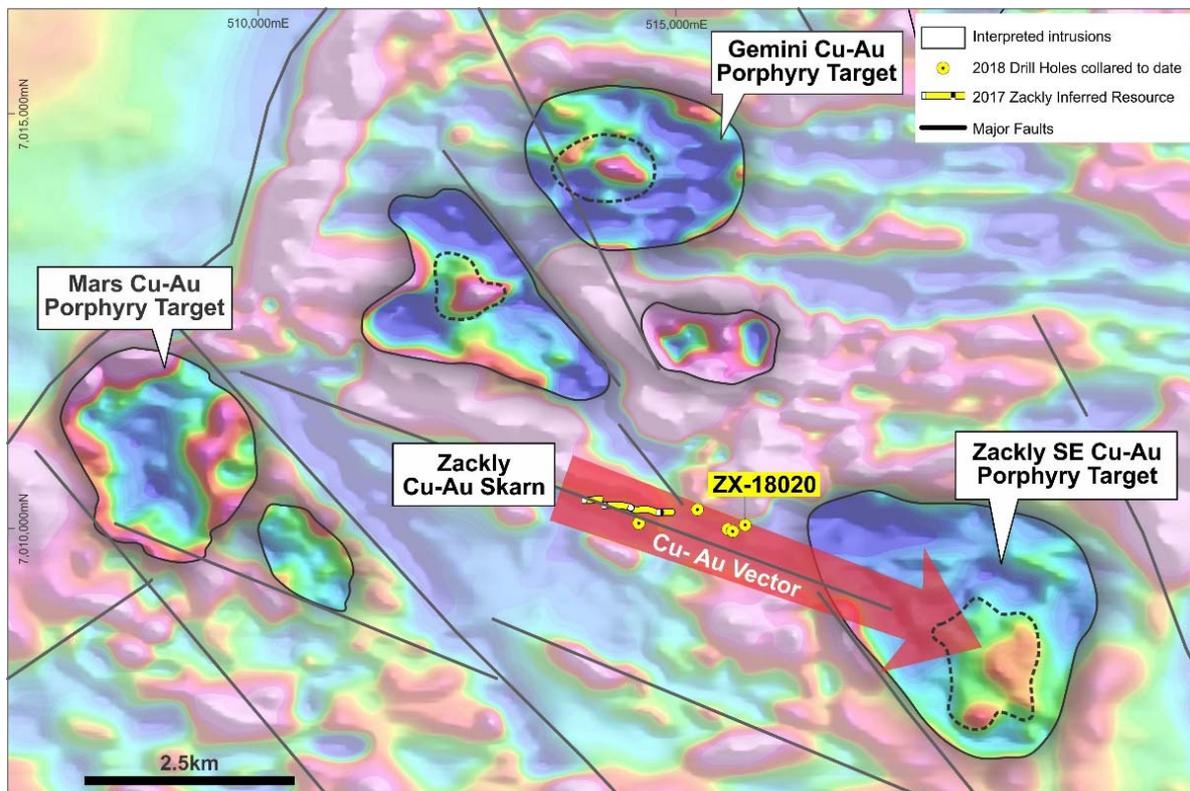
**Figure 4** Aeromagnetic imagery showing a prominent magnetic anomaly to the SE of the Zackly inferred resource. **Note the recently completed drill hole ZX-18020 in which thick zones of gold and copper mineralisation were intersected in association with quartz-sericite alteration, suggesting a possible vector of increasing widths of mineralisation towards the magnetic anomaly which represents a porphyry Cu-Au target.**
