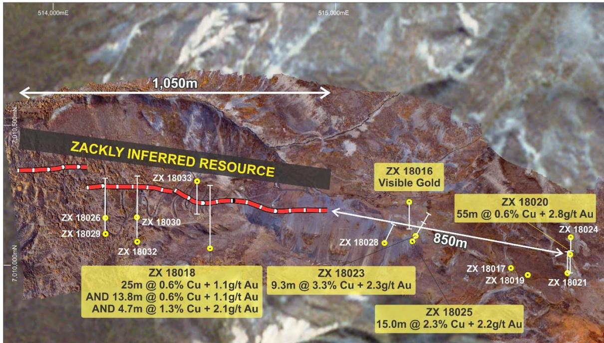
Figure 2. Drill hole plan for Zackly showing the 2017 surface trace of PolarX's inferred resource outline (red) and the 2018 drill holes collared to date (yellow) on detailed drone imagery.
