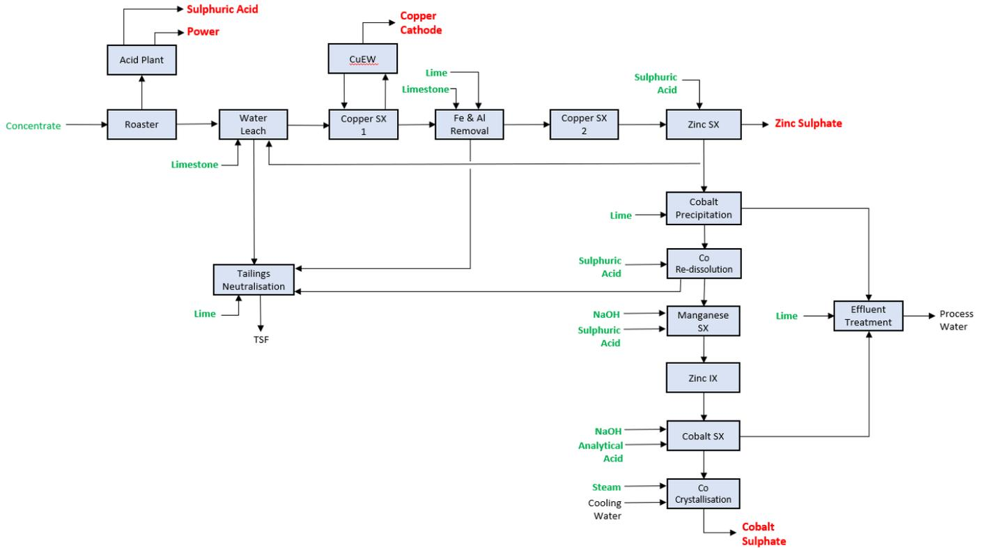
**Figure 4: Preliminary Autoclave Leach Option Flowsheet**
