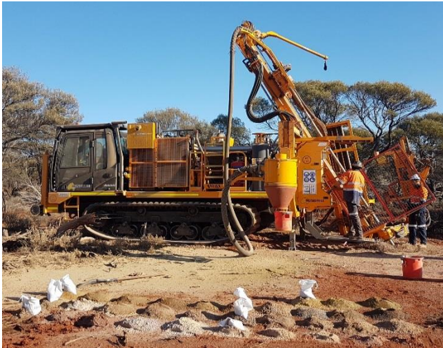
Ausdrill aircore rig onsite at Redcliffe
