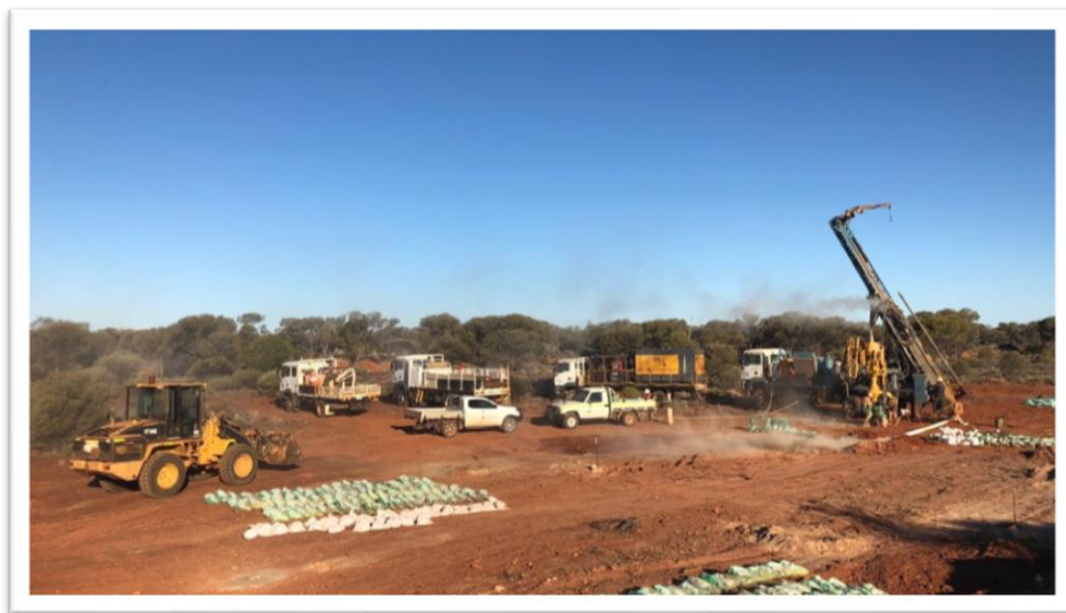
Figure 2. RC drilling at the Southwark deposit, Bottle Creek.
