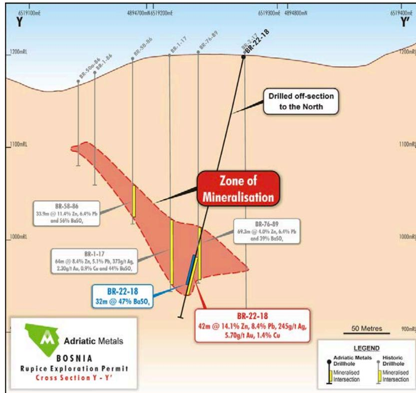
Figure 3: Cross Section illustrating drill hole BR-23-18
