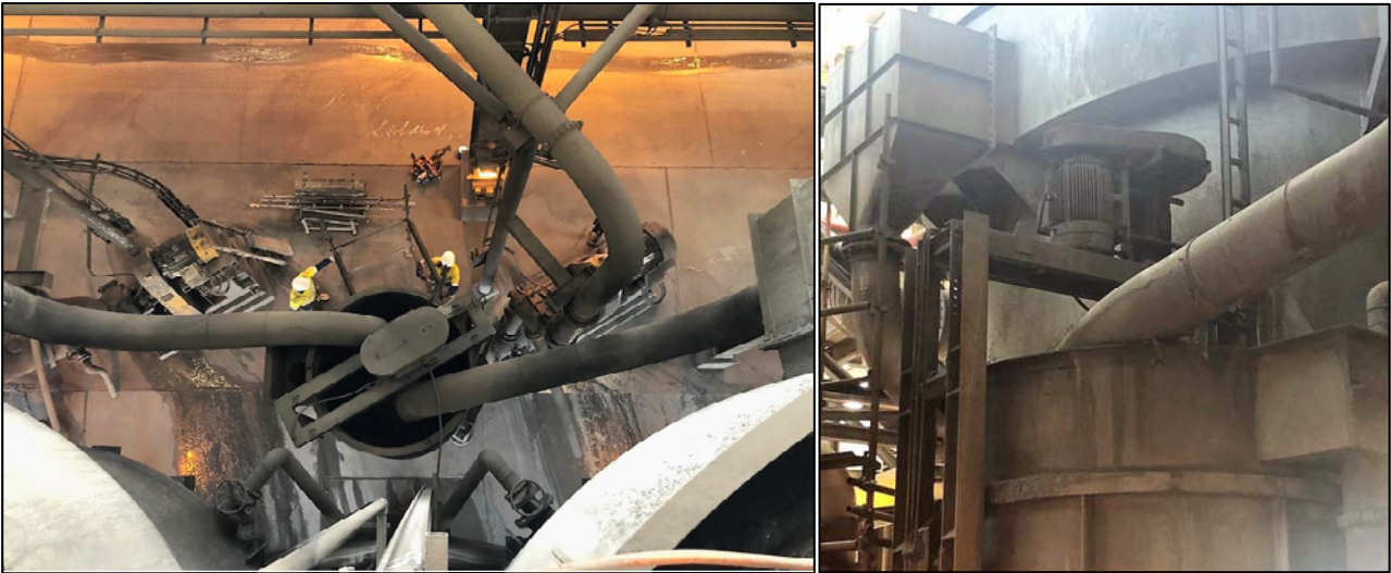
Figures 6 & 7: Top view (left) and side view (right) of the existing mechanical 'froth bashers' now undergoing refurbishment. The froth bashers breakdown bubbles entering in the interstage pumping feed tanks, assisting to reduce the froth associated with the floated concentrate to a pumpable liquid
