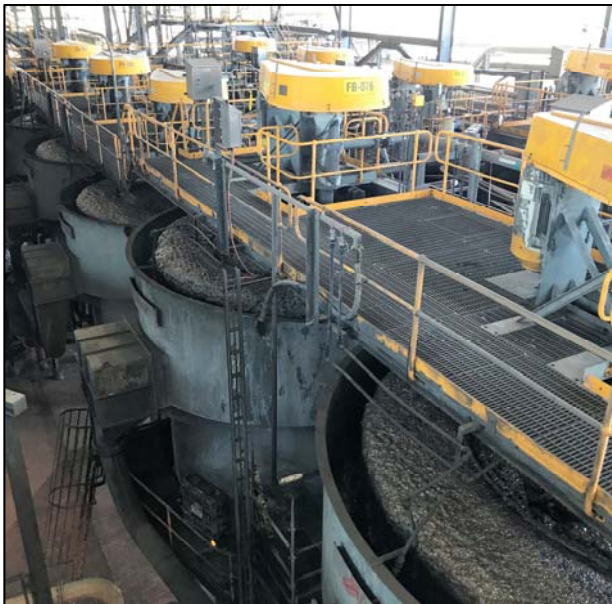
Figures 2 & 3: Rougher/scavenger flotation (left) & production of cleaner circuit concentrate (right)
