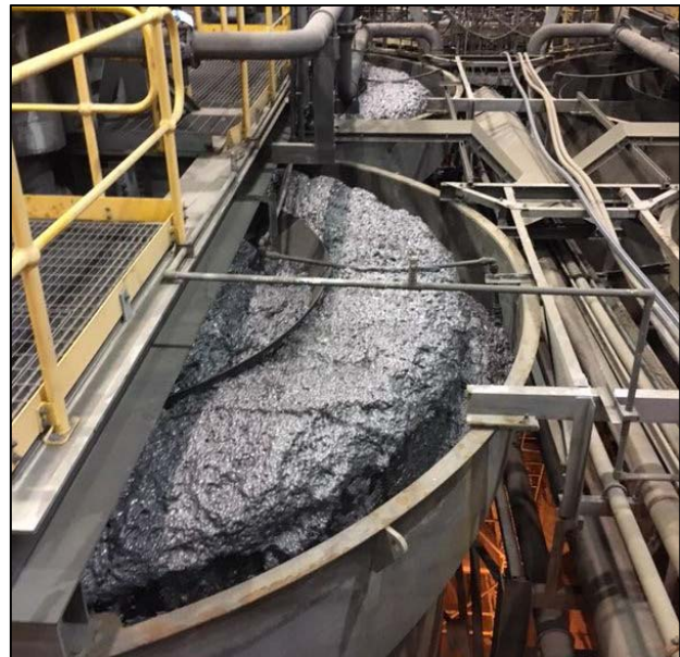
Figures 2 & 3: Rougher/scavenger flotation (left) & production of cleaner circuit concentrate (right)
