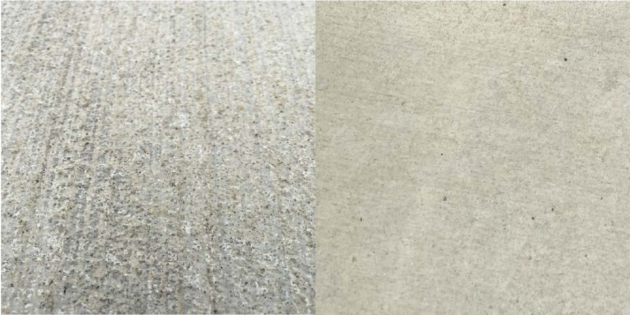
Figure 2: MARTA Brady Facility – Reference slab showing significant abrasion (Left) and EdenCrete® slab showing minimal surface abrasion (Right) in the same period of time
