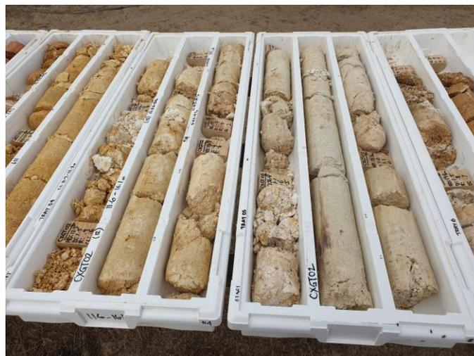
Selected Diamond Core Samples (PQ) from Geotechnical Hole CXGT02
