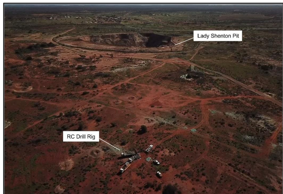
Figure 1: Reverse Circulation drill rig (foreground) completing pre-collars for deep diamond drilling at Lady Shenton deposit (open pit in background).
